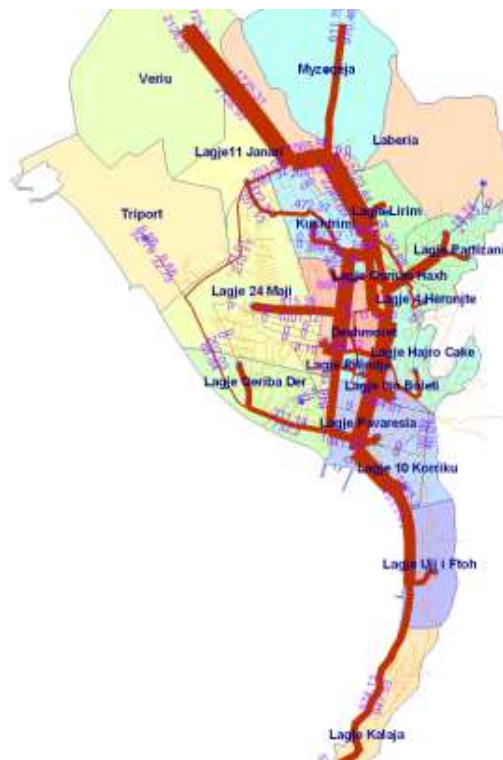
Figure 2 Introduction of traffic fluxes over the road network of urban space in city of Vlora with method “all or nothing”, realized with TRANSCAD for year 2030
