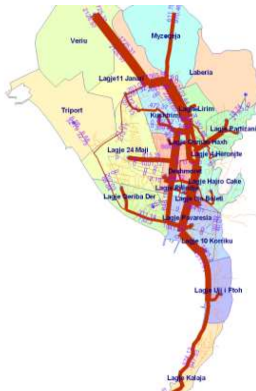
Figure 1 Introduction of traffic fluxes over the road network of urban space in city of Vlora with method “all or nothing”, realized with TRANSCAD for year 2012
