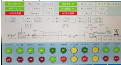
Figure 6 PET sheet line control system [11]
