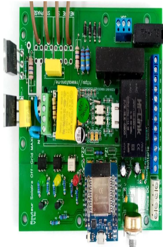
Figure 6 Off grid system to maximize photovoltaic self-consumption [7]
