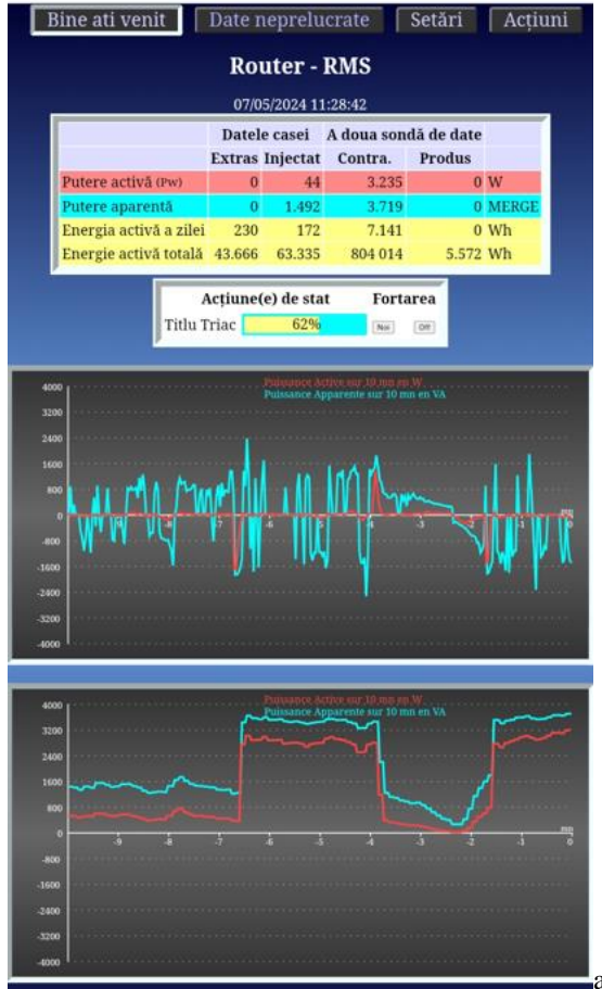
Figure 4 a) Active triac dimming with input-output load 2400W
