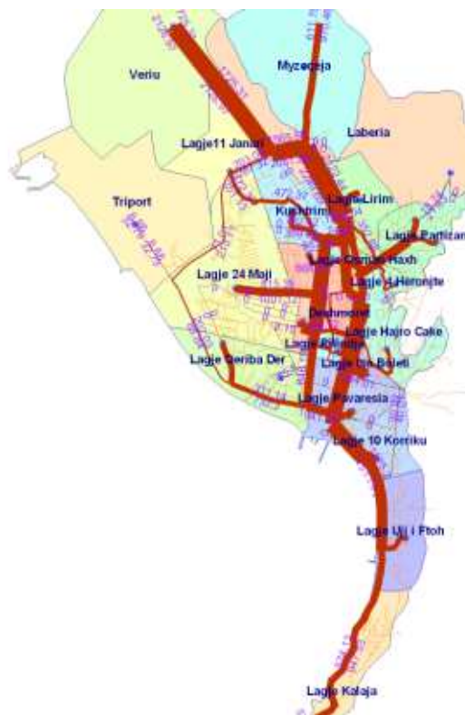
Figure 1 Introduction of traffic fluxes over the road network of urban space in city of Vlora with method “all or nothing”, realized with TRANSCAD for year 2012
