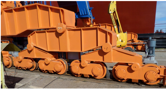
Figure 6 Motion system of the crane, leg no. 3
