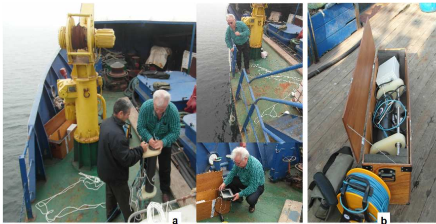
Figure 2 Images capture from the measurements campaigns, where: a) preparations of the instruments and measurements; b) overview of the system Midas 808-400
