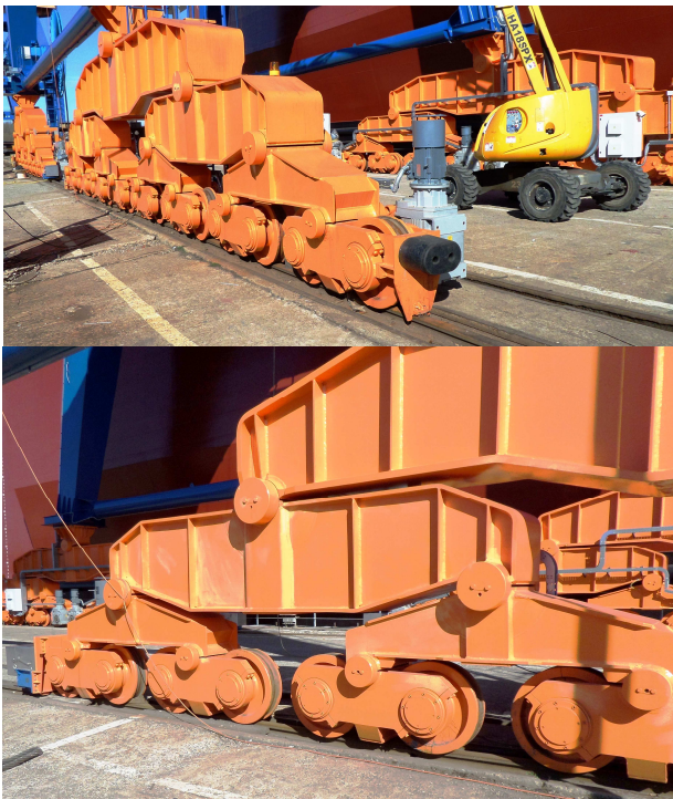
Figure 4 Rail mounted quay crane
