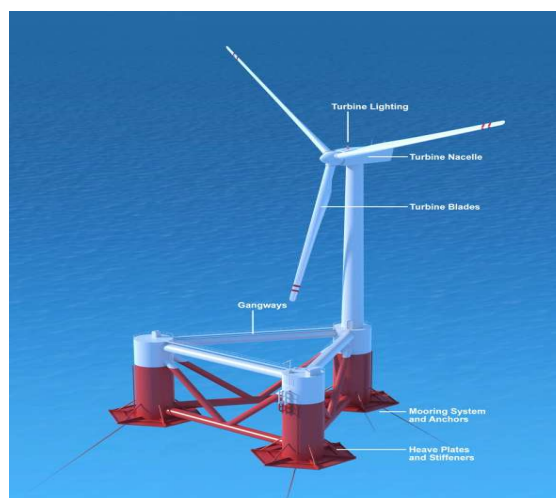
Fig. 1 Floating wind turbine [2]
