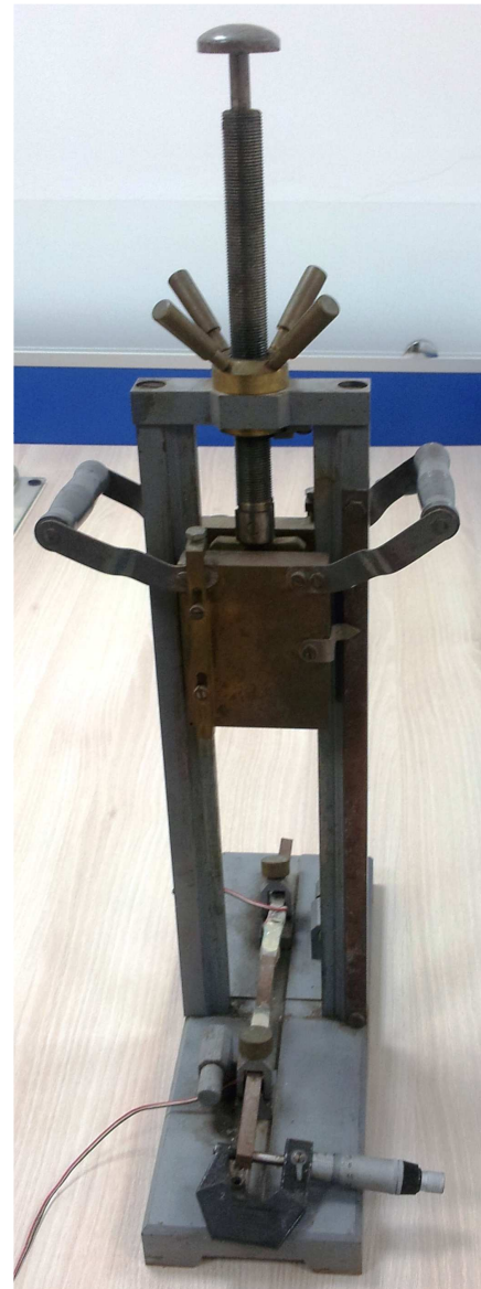
Figure 5 – Device which was initially designed to measure the effects of a shock loading
