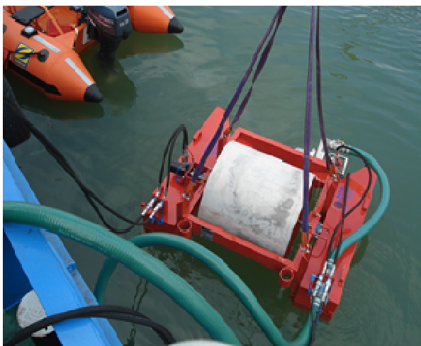
Figure 2 The skimmer from Danube Eco 1 ship
