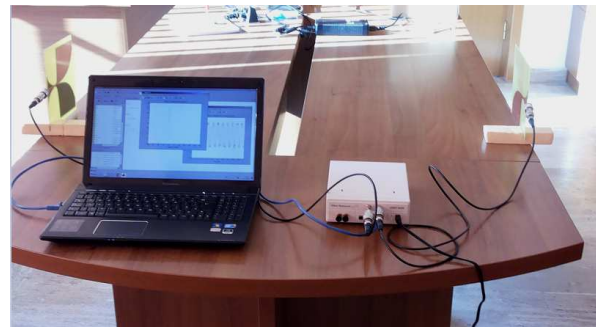
Figure 6 Software Defined Radio (SDR) arc locator – practical implementation
