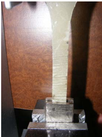
Figure 6. The first cracks specimen two.
