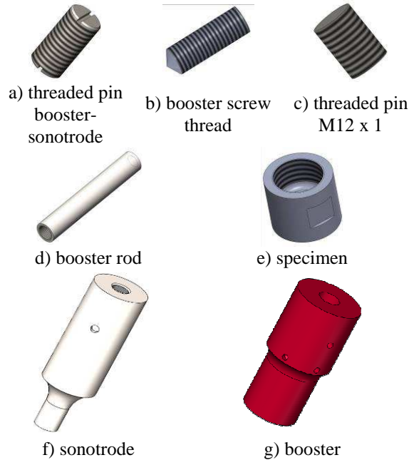
Figure 4 Component elements of the booster-sonotrode-specimen assembly
