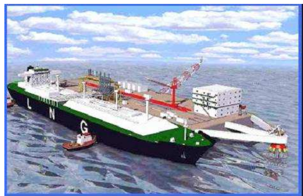
Figure 1: Floating Storage Regasification Unit (FSRU)
