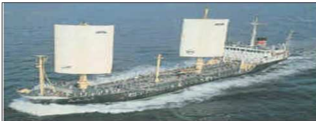
Figure 3 Tanker “Shin Aitoku Maru”, the first modern ship equipped with rigid sails
