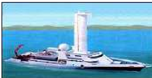
Figure 4 The ship "Calypso" equipped with Turbo sails
