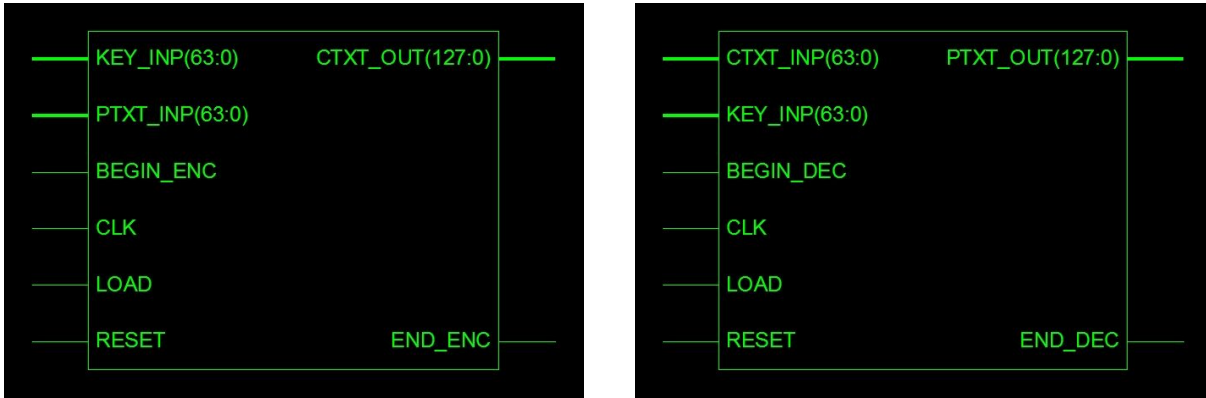
Figure 4. The encryption/decryption blocks of AES-128
