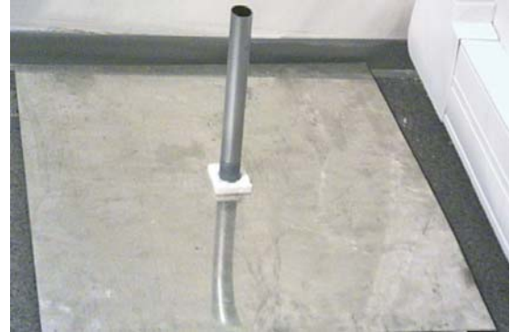
Figure 3 Cylindrical monopole. Antenna dimensions: rod length=22.5 mm, rod diameter=25 mm, gap length =5mm, ground plane side length = 500 mm
