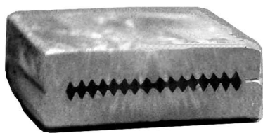
Fig. 3.2 Cold welded samples with intermediate cogged layer
