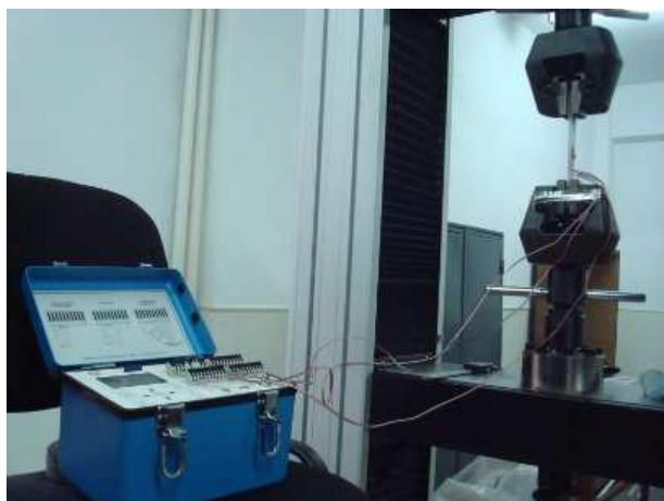
Figure 3 The apparatus for the tensile tests
