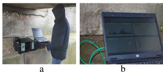
Figure 3 Determination of vibration values of the marine environment when sampling: a - an overview of the equipment used, b - recording the vibrations on the laptop screen
