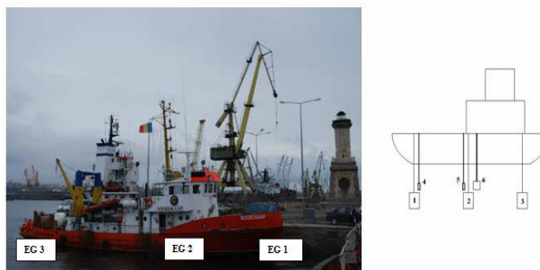
Figure 4 The « Noordkaap » ship and the cages location 1, 2, 3 –the cages with experimental groups; 4, 5 – hydrophones; 6 –the source of noise
