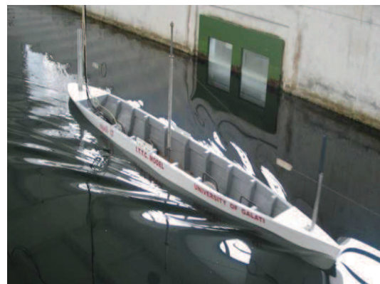
Fig.1.1a Free surface topology to confirm the numerical simulation by pool tests.
