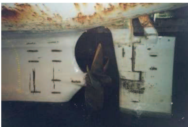
Figure 3 Sacrificial anodes on the ship's hull [1]
