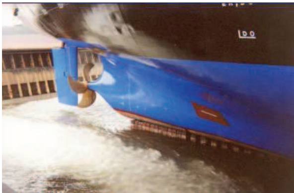
Figure 7 The anode in ICCP system [1]
