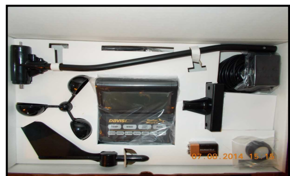
Figure 2 Parts of the portable automatic weather station type "DAVIS"
