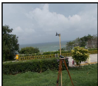
Figure 1 Placement of the portable weather stations type "DAVIS" (station A, and B)
