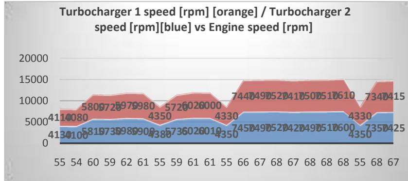
**Fig. 4.11** Turbocharger speed vs engine speed
