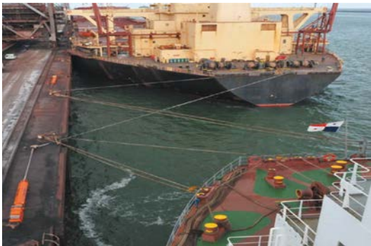
Figure 4 Shore Tension System securing the ships
