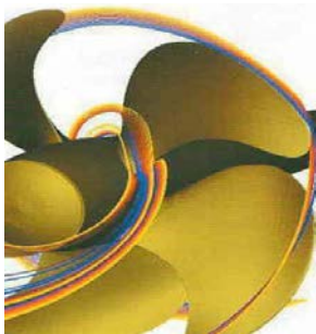
Figure 1 Escher Wyss Controllable Pitch Propellers with calculated streamlines
