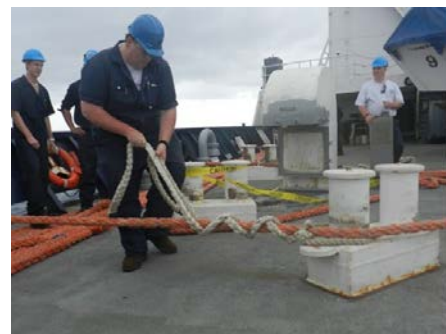
Figure 5 Making fast the line on the bollard- dangerous movement
