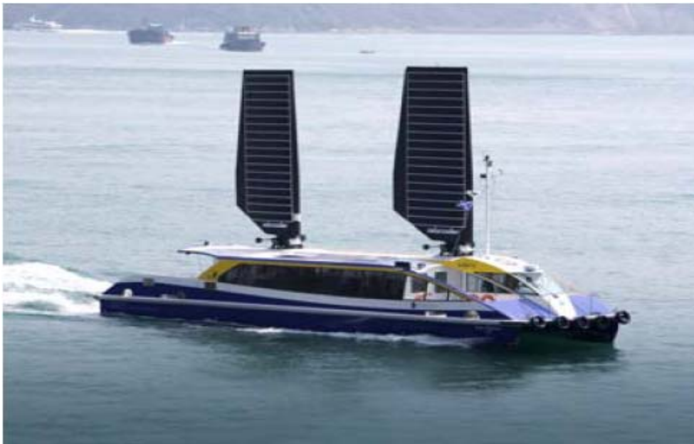
Figure 6 Ship that harnesses solar energy and wind energy
