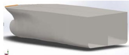
Figure 3 Execution stages for the three dimensional model. 3d. Bow section [2]
