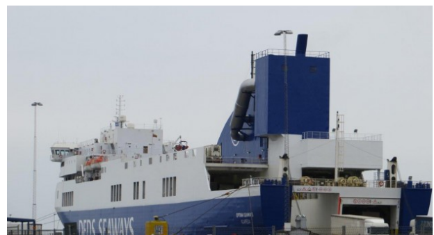
Figure 4 OPTIMA SEAWAYS with its newly installed scrubber, which is located behind the existing funnel casing
