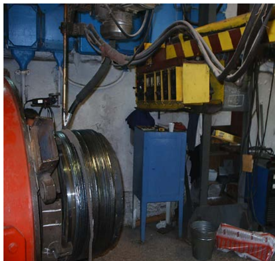
Figure1. Welding of the piston head under a layer of flux
