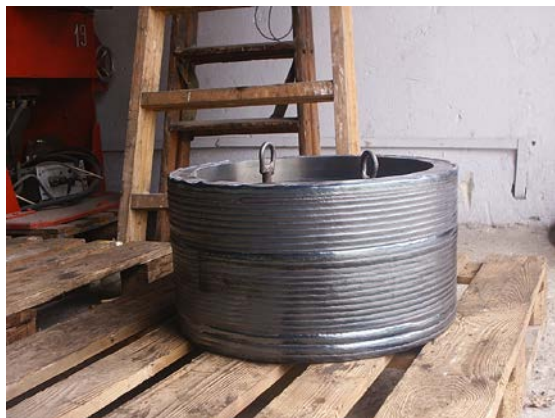
Figure 3 Completed welded part
