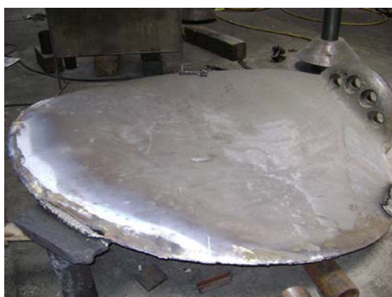
Figure 6 Building up missing sections
