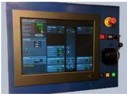
Figure 9 Modern Flettner Rotor Controls
