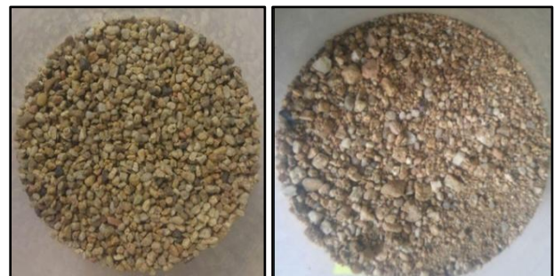
Figure 5 The samples of homogeneous and inhomogeneous sand
