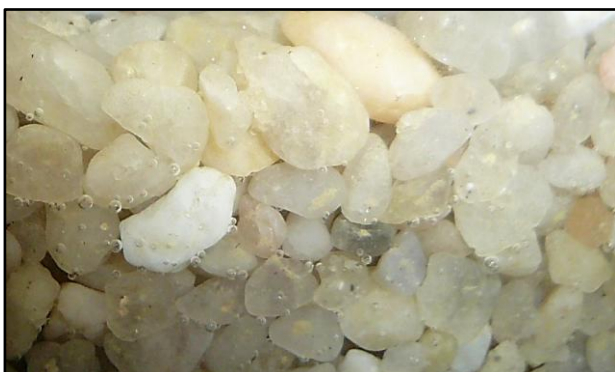
Figure 4 Air bubbles when measuring a soil sample loaded with distilled water
