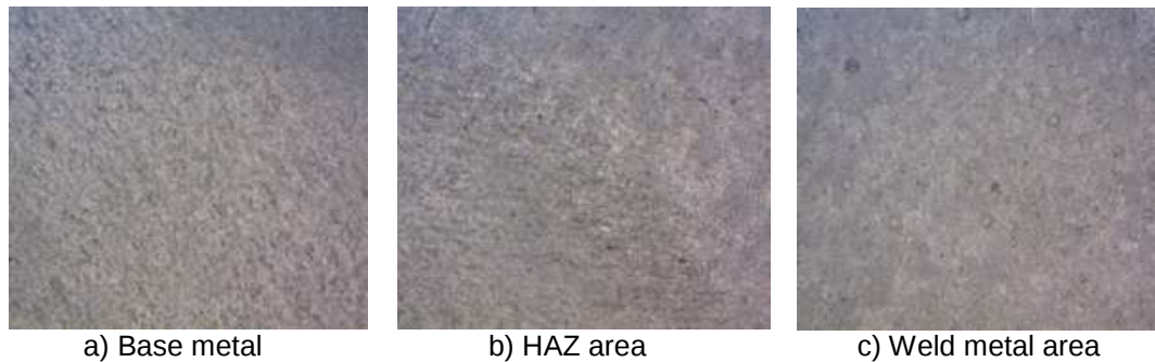
Fig. 5. Microstructure for MIG specimens (200x magnification)
