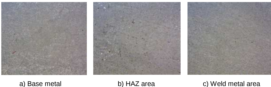
Fig. 4. Microstructure for TIG specimens (200x magnification)
