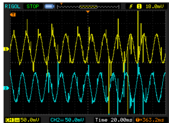
Figure 9 Oscilloscope of phase currents in phase V and phase U. Yellow signal - I_{UN} ; blue signal - I_{VN} . Set frequency of the output voltage – 50 Hz, set PWM frequency – 10 kHz
