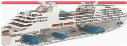
Figure 1 General layout of electrical power equipment and substations of cruise ship
