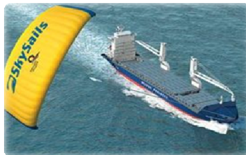
Figure 3 M/V Beluga powered by a kite from Sky Sails
