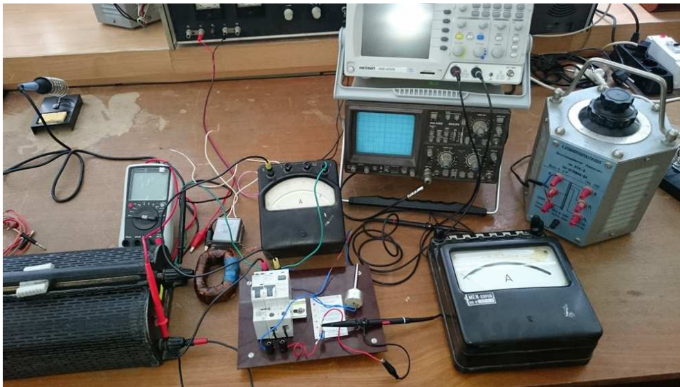
Figure 4 General view of the elaborated laboratory stand with the measuring instruments and the load
