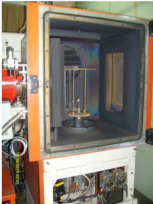
Figure 1 General view of the engine, used for the deposition of TiN coatings on low voltage busbars
