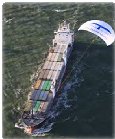
Figure 4 M/V Beluga powered by a kite from Sky Sails
