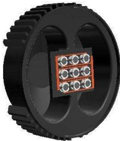
Fig. 5 Structure of the system LED matrix – cooling body.
