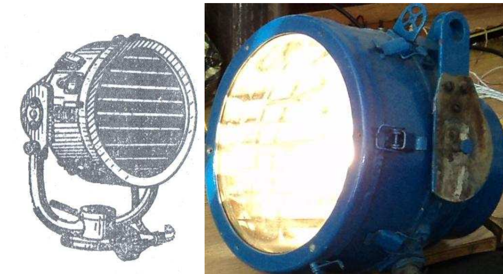
Fig. 1. Sketch and photo of the investigated searchlight type MSNP-250M
