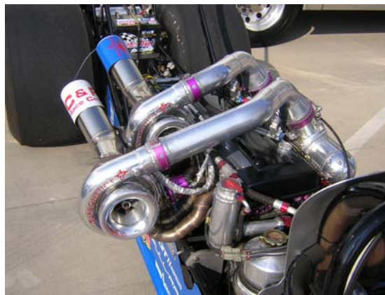
Fig.2. A pair of turbochargers mounted to an Inline 6 engine (2JZ-GTE from a MkIV Toyota Supra) in a dragster.
