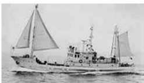
Fig.4: Soft Sail, Japan Fisheries Boat, 1985
