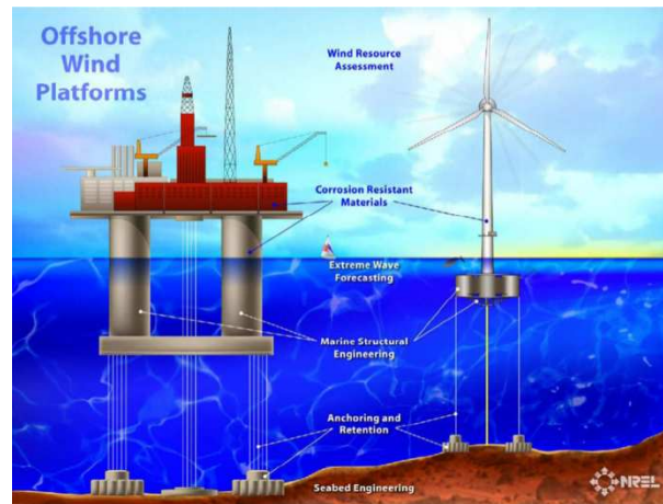
Fig. 3. Synergies between offshore petroleum industry and wind structures SOURCE: NREL
