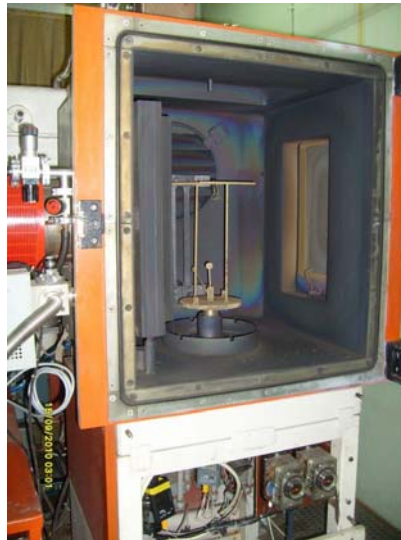
Fig. 1 General view of the engine, used for the deposition of Ti/TiN nanostructured coatings on rivets of electrical contacts
