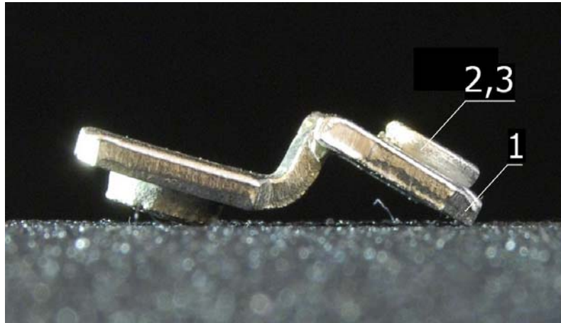
Fig. 4 General view of electrical contact with nanostructured multilayer coating on the contact body. 1 - conductive plate, 2,3 - contact body with the nanostructured coating
