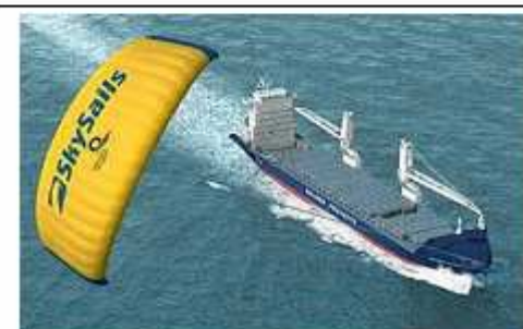
Fig.8: Kite sail, Preliminary Design, SkySail, 2007
