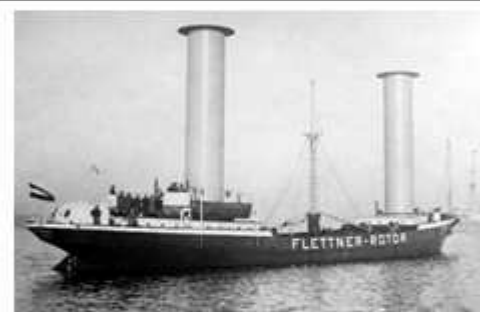
Fig.6: Rotor sail, Germany, 1924
