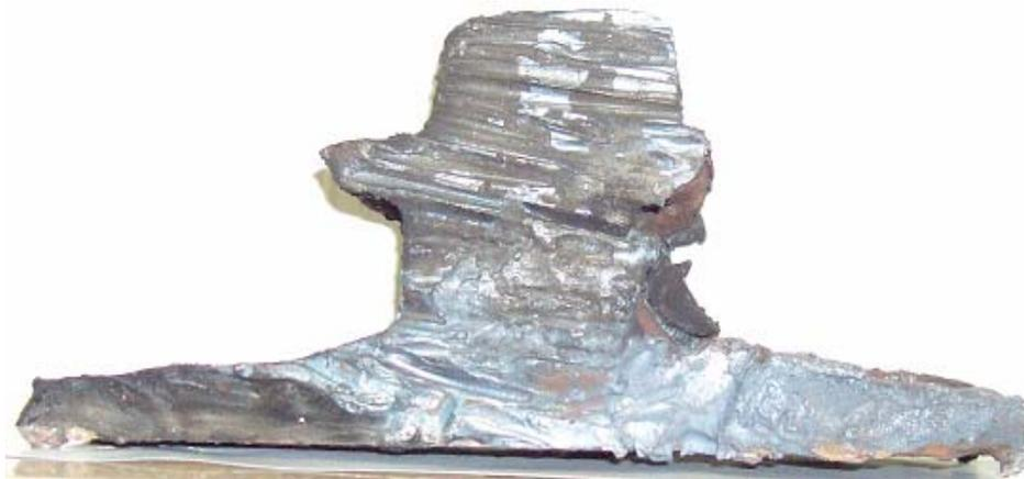
**Fig. 1. Wear out rail after many years of exploitation**
