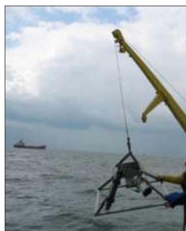
Fig. 3.2. Mounting of the ADCP WH600 on a non-magnetic metallic structure, in a wide station
