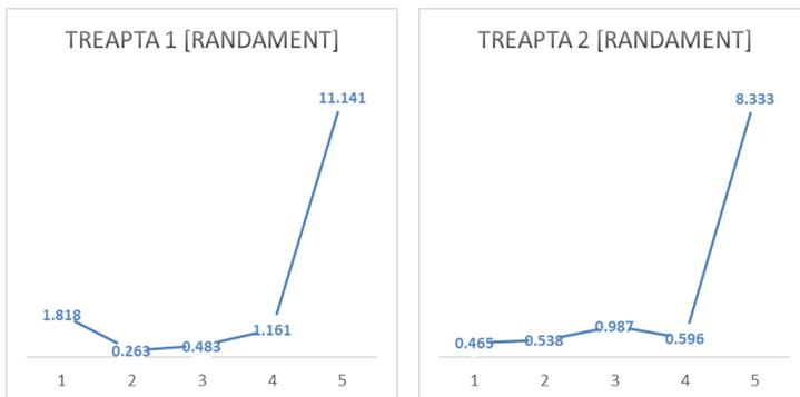
Fig. 4.19. Graph measurement results for the efficiency [  $\eta$  ] of non-conventional naval thrusters
