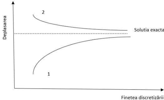
Fig. 5.5. The influence of the number of elements (nodes) on the accuracy in CFD analysis
