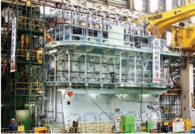
Fig. 2.1. Slow diesel engine (Wärtsilä RT-flex82T version B, main engine) [28]
