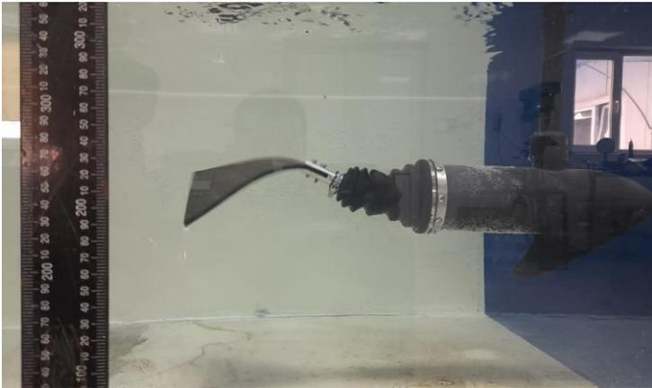
Fig. 4.10. Measurement of pala\_z movement amplitudes (test 1)
