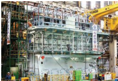
Fig. 2.1. Motor diesel lent (Wärtsilä RT-flex82T versiunea B, motor principal) [28]
