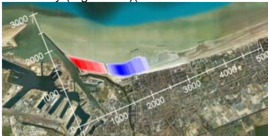
Figure 6.2. Examination of beach nourishment at Dunkeque Port, France. Red colours indicate erosion. Source: Grunnet et. al. 2012
